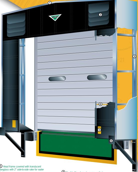
1 Head frame covered with translucent fiberglass with 2" side-to-side rake for water drainage.
