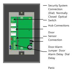
Module Connection 12 VDC Switch Signal Interior Panic Alarm (K11967CRH0A7)
