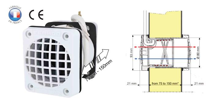
The F2227 Valve makes it possible to balance internal & external pressures through venting. It's mechanically operated valves (one intake and the other exhaust) has two watertight mobile flaps. This means that when not required the cold room is still sealed without precious cold air leaking out of the room and causing machinery to run more often. When pressure builds up the valves open and allow equalisation.
