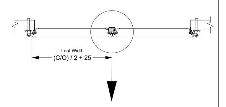
Center Rebate has 2 flush bolts and is injected with polyurethane
