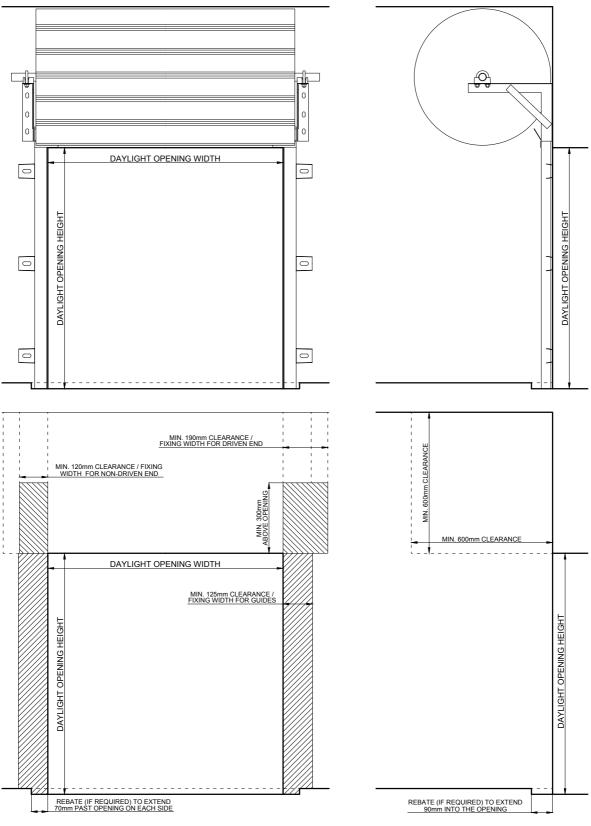
• All fixing surfaces must be flat and flush.
