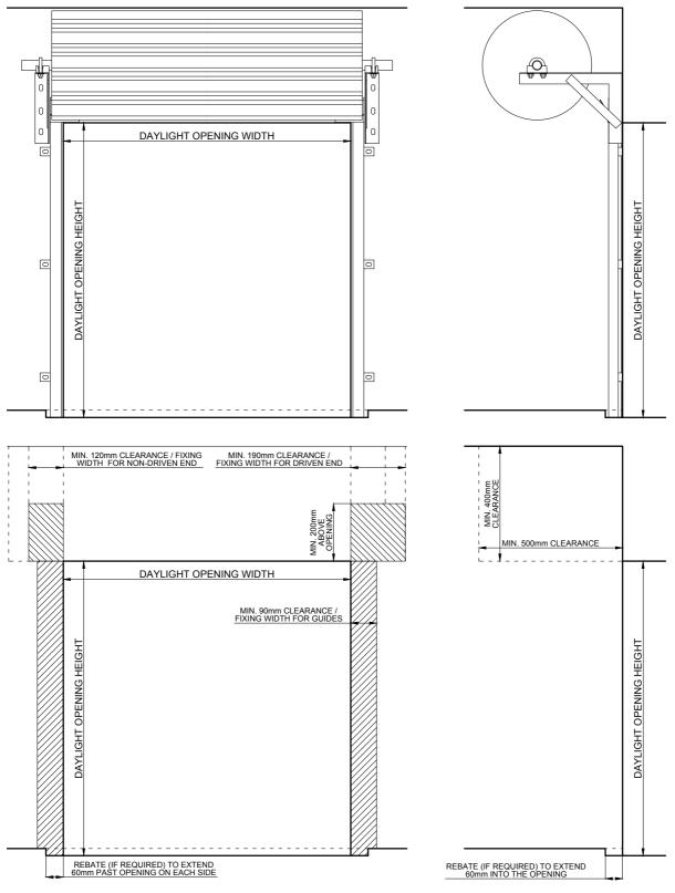
• All fixing surfaces must be flat and flush.
