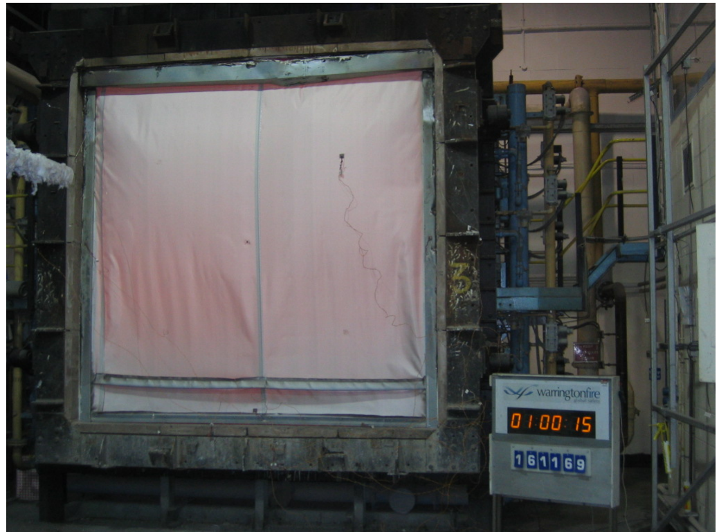
The unexposed face of the specimen after 60 minutes of testing
