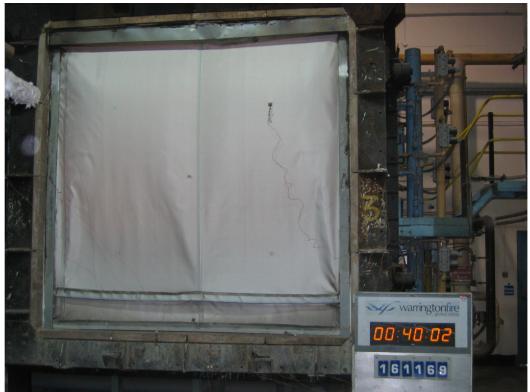
The unexposed face of the specimen after 40 minutes of testing
