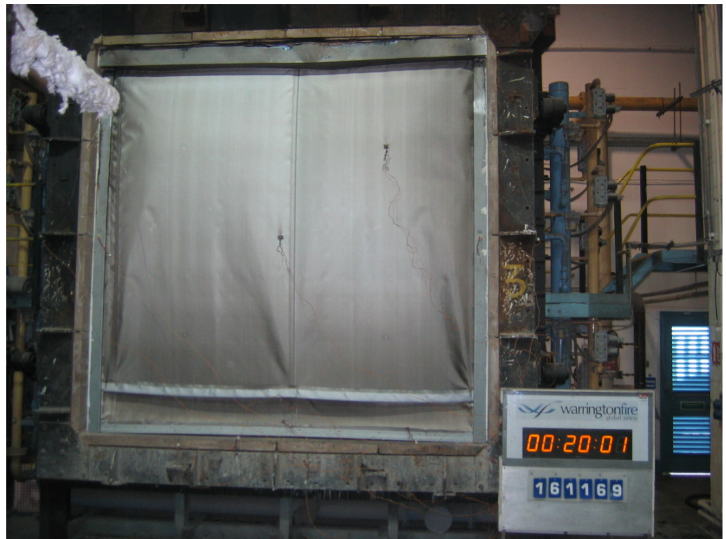
The unexposed face of the specimen after 20 minutes of testing
