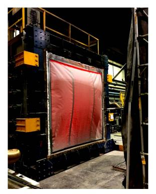
Kent Automatic Fire Curtains create physical barriers against the passage of fire. They remain virtually invisble when the curtain is stored in its retracted position within the compact headbox. When signalled by a local detector device or a fire alarm signal, they descend safely to the floor to provide up to 180 minutes of fire resistance.
